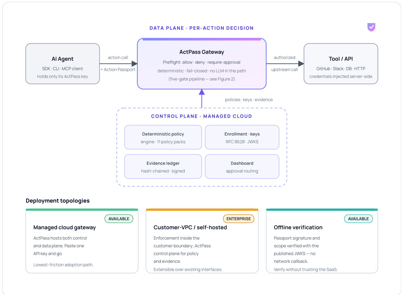
Figure 1. The agent calls the ActPass gateway (data plane), which renders the preflight decision and optionally proxies to the tool; the control plane owns policy, keys, ledgers, the credential vault, and evidence, feeding the data plane cacheable bundles and receiving evidence asynchronously — shown across the managed-cloud, customer-VPC, and offline-verification placements.
